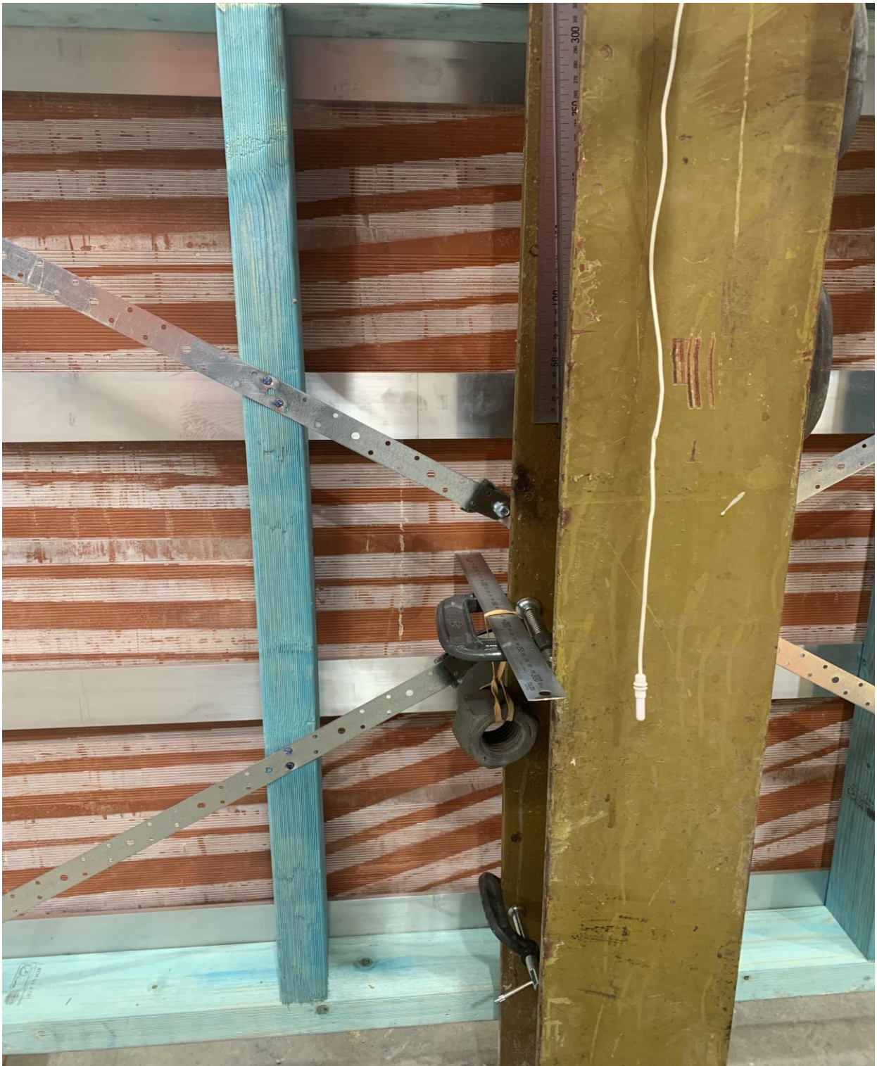
PHOTOGRAPH 2 - Soft Body Impact Test - Deflection Measurement - Note the steel rule
