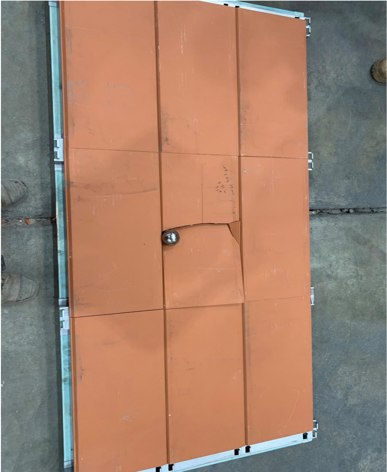
PHOTOGRAPH 3 - Hard Body Impact Test - Typical Panel after test
